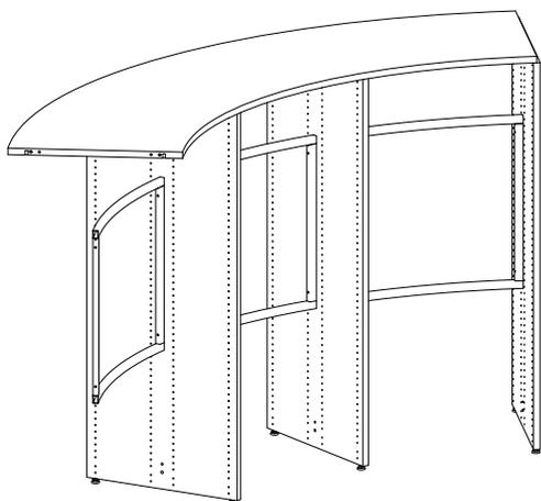
An intermediate section starts without an intermediate panel and ends with an intermediate panel.
