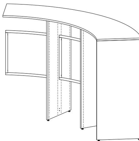
The right starter section starts with a right end panel and ends with an intermediate panel.
