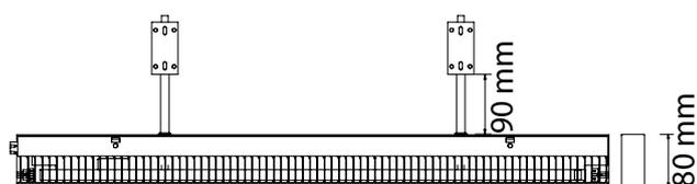
Model showing 2 bearing arms incl. light tube and louvre. Armature housing in aluminium.
