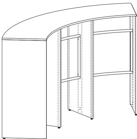
The left starter section starts with a left end panel and ends with an intermediate panel.
