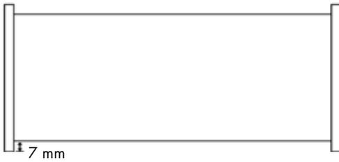
The distance between the front edge of the end panel and the front edge of the shelf is 7 mm. The shelves are adjustable in 25 mm increments.
