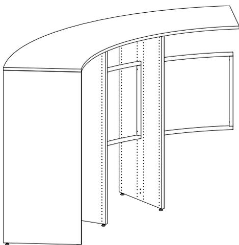
The left end section starts without an intermediate panel and ends with a left end panel.
