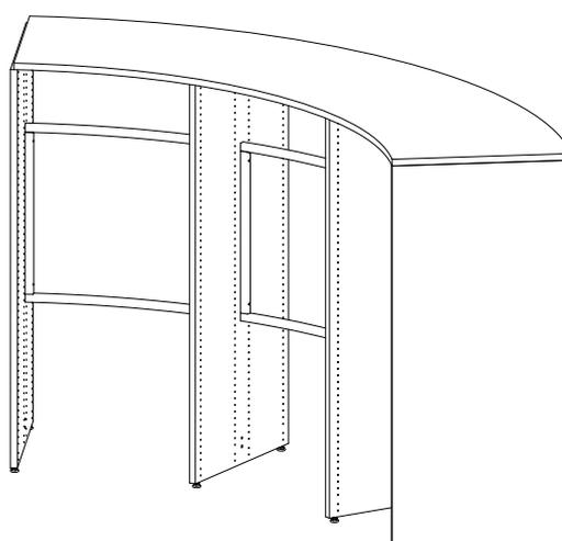
The right end section starts without an intermediate panel and ends with a right end panel.
