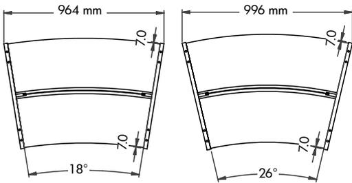
The distance between the front edge of the end panel and the front edge of the shelf is 7 mm. The shelves are adjustable in 25 mm increments.
